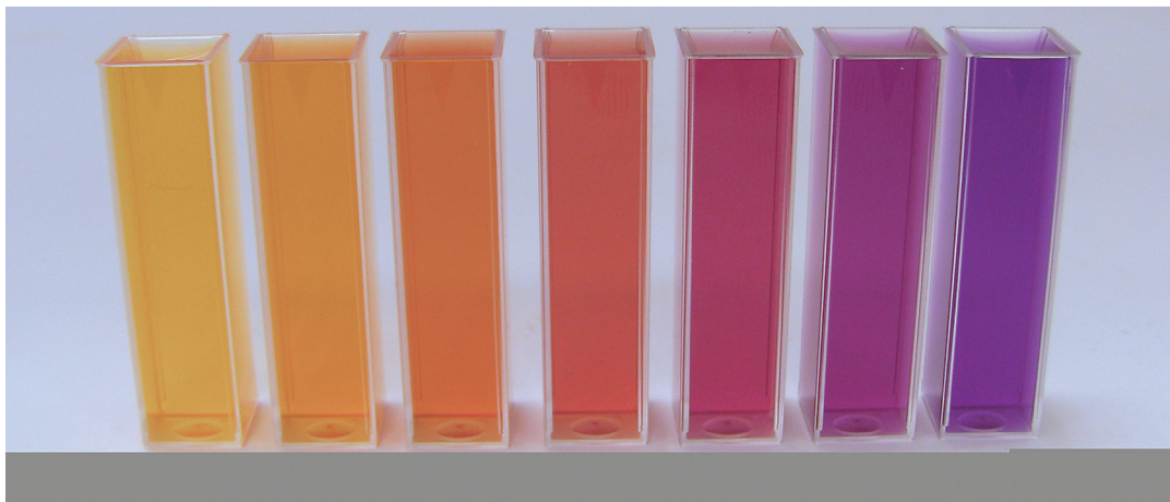
Figure 1 Hydrogencarbonate indicator solutions in the range pH 6.8 (pale yellow) to pH 9.2 (purple); pH increases in increments of 0.4 units
