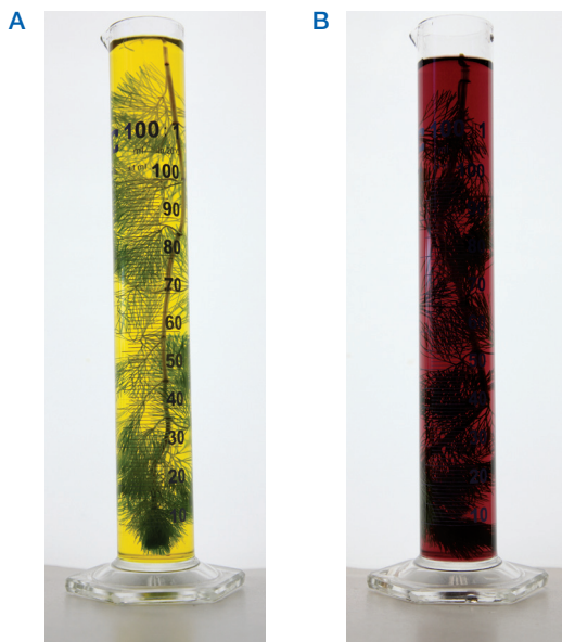
Figure 3 Effect of irradiation on Cabomba /hydrogencarbonate mixtures: (A) after 4 hours of irradiation during which the cylinder was covered in black paper (pH measured to be 6.8); (B) after 4 hours of irradiation (pH measured to be 8.3)
