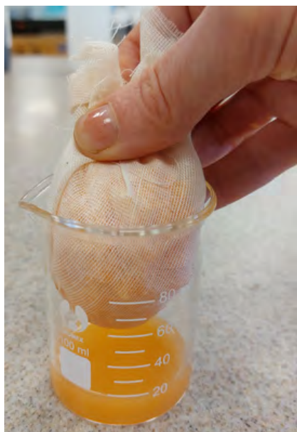
Figure 4: This procedure allows the extraction of beta-amylase (enzyme) from sweet potato. A 30 g sample of sweet potato is cut, blended and then passed through muslin. The collected liquid contains the enzyme and can be stored.
