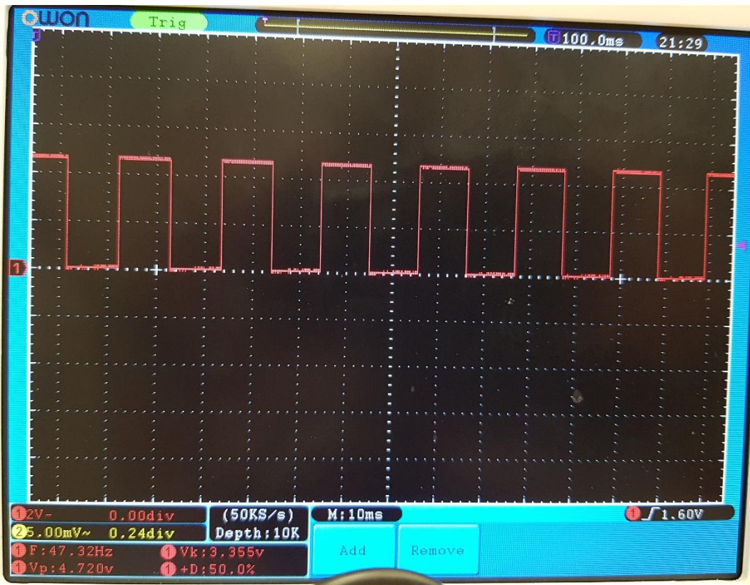
Fig 8. Pulsed (TTL) waveform. Fixed 5 V 50% duty cycle.
