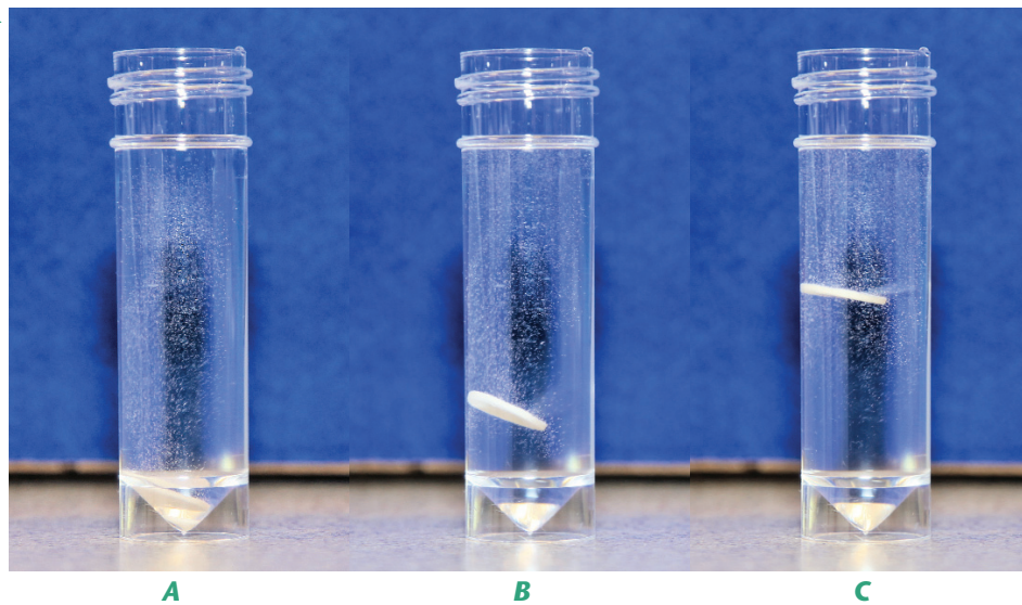
Figure 1 - A single drop of a 1% suspension of yeast has been added to a filter disc and then placed in a 1% solution of hydrogen peroxide. Photographs were taken at (approximately) 3 s (A), 8 s (B) and 13 s (C).
