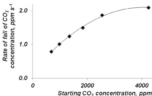
**Figure 8** The rate of fall of CO<sub>2</sub> concentration in the chamber as a function of initial CO<sub>2</sub> concentration
