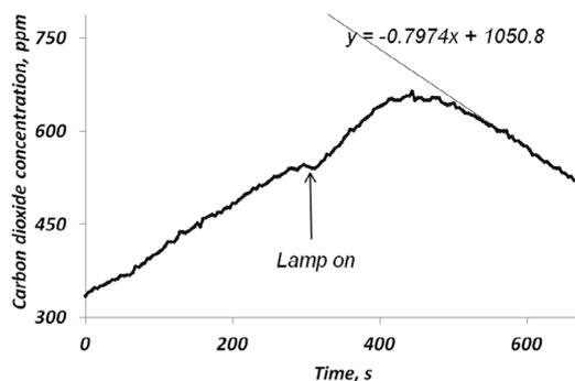
**Figure 7** The CO<sub>2</sub> concentration in the chamber as the experiment progressed
