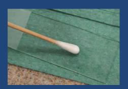
Smear the cotton swab over 2 a small area of a clean microscope slide. Place the used cotton bud immediately in a small volume of freshly prepared disinfectant.
