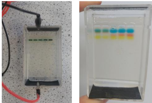
**Figure 4:** Electrophoresis tank set up with carbon fibre electrodes, each connected to the power supply. 10 µl of each sample are loaded into the wells. Electrophoresis should continue at 36 V for 20 minutes. The result shown on the right could be used to demonstrate that Suspect 1 (well 2) matches the "DNA" sample obtained from the crime scene (well 1). Alternatively, akin to the original "Wizard Genes" protocol, the gel results could be used to determine the powers of each wizard.
