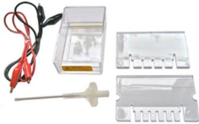
The “base unit” consists of all the re-usable parts required for gel electrophoresis, except for the [36 V transformer](#). The “base unit” contains 8 sets of the equipment, i.e.
